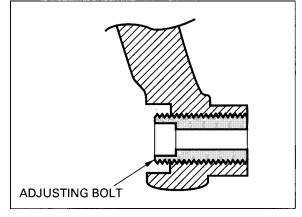
Install the rear/lower engine hanger bolt.
