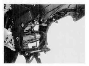
Install the engine hanger adjusting bolts so that the adjusting bolts does not projected inside surface of the frame.
