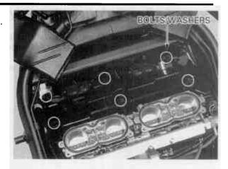
Remove the cylinder head cover forward.
