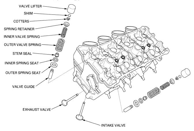
Clean the cylinder head assembly with solvent and blow through all oil passages with compressed air.
