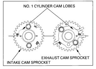
Clean and apply a locking agent to the cam sprocket bolt threads.
