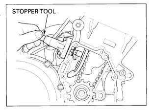
Remove the bolts, sealing washers and cam chain tensioner lifter.
