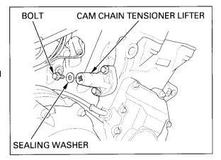
Turn the tensioner shaft fully in (clockwise) and secure it using the stopper tool to prevent damaging the cam chain.
