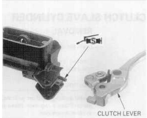
Install and tighten the pivot bolt to the specified torque.
