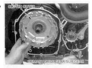
Install the washer onto the clutch outer.
