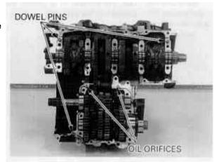
Install the lower crankcase onto the upper crankcase.
