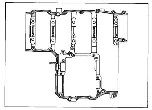
Install the three dowel pins.
