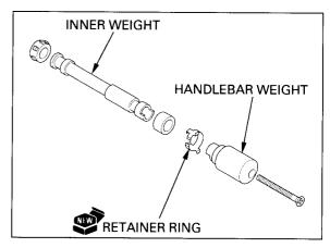
Insert the handlebar weight assembly into the handlebar.
