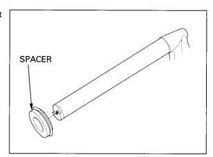
Apply Honda Bond A or equivalent to the inside of the grip and to the clean surfaces of the left handlebar and throttle grip.
