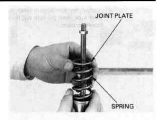
Pour out the fork fluid by pumping the fork tube up and down several times.
