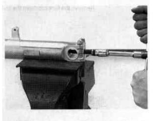
Remove the fork damper assembly and oil lock piece from the fork tube.
