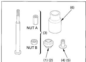
Install the ball race remover into the head pipe as shown.
