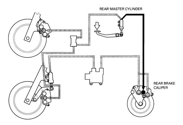
5. Feed the brake fluid at the rear brake caliper center bleeder valve as same procedure in step 1.
