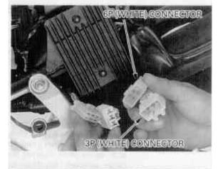
If the regulated voltage reading (see page 16-6) is out of the specification, measure the voltage between connector terminals (wire harness side) as follows:
