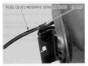
Remove the nuts and fuel level sensor/reserve sensor unit from the fuel tank.
