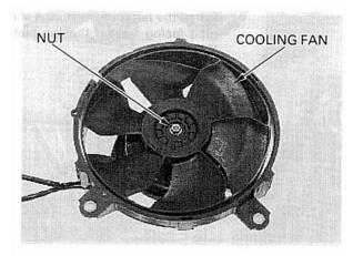
Remove the three bolts and the fan motor from the shroud.
