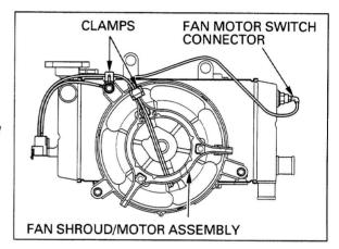
Remove the nut and cooling fan from the motor.
