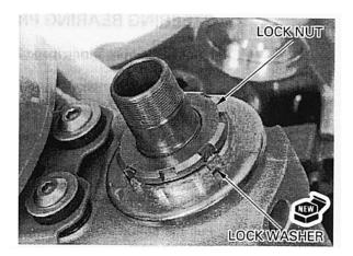
Install the fork top bridge and steering stem nut. Temporarily install the forks into the fork bridges. Tighten the steering stem nut.
